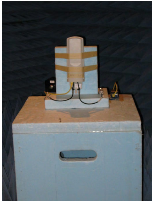
Radiated from Cabinet Above 1 GHz - Front
