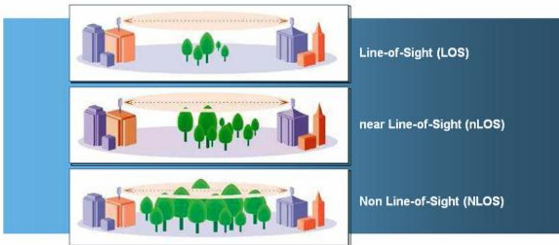
Whereas multi-pathing degrades a link in some technologies (FSK, for example), OFDM can often use multi-pathing to an advantage to overcome nLOS, especially in cases where the Fresnel zone is only partially blocked by buildings, “urban canyons”, or foliage. OFDM tends to help especially when obstacles are near the middle of the link, and less so when the obstacles are very near the SM or AP.
