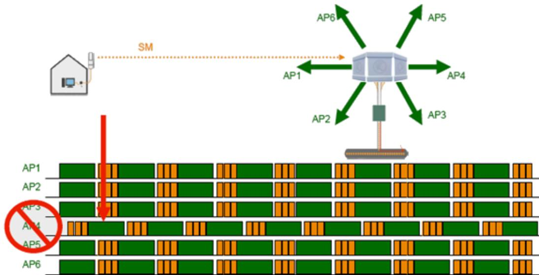
The result is self-interference. In this scenario, the self-interference can be avoided only by synchronizing the TDD transmit cycles of all APs that operate in the same frequency band.
