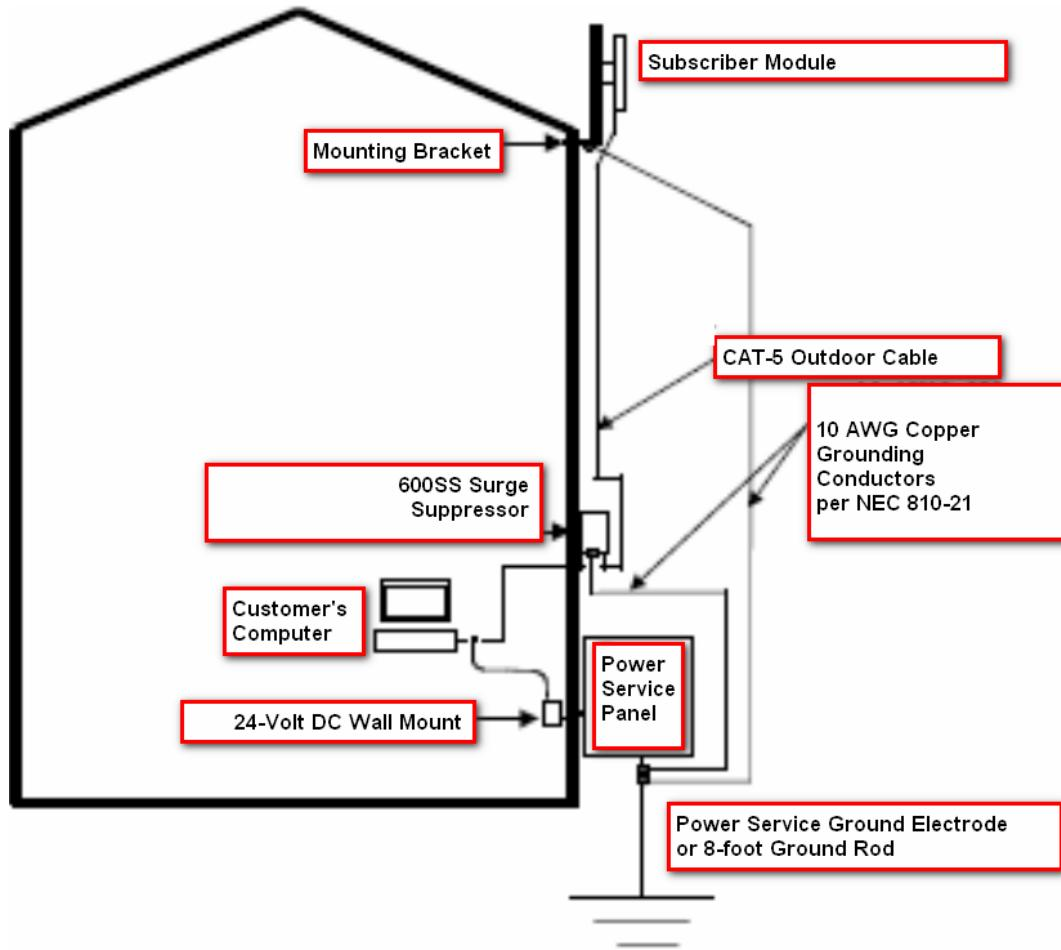
**9** Wrap an AWG 10 (or 6mm<sup>2</sup>) copper wire around the Ground post of the 600SS.
