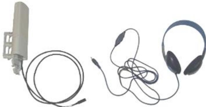
Adjust the module slightly until you hear the highest pitch and highest volume.
