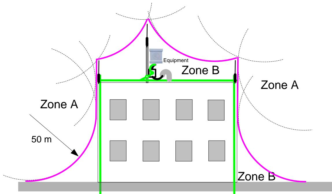
Assess locations on masts, towers and buildings to determine if the location is in Zone A or Zone B:
