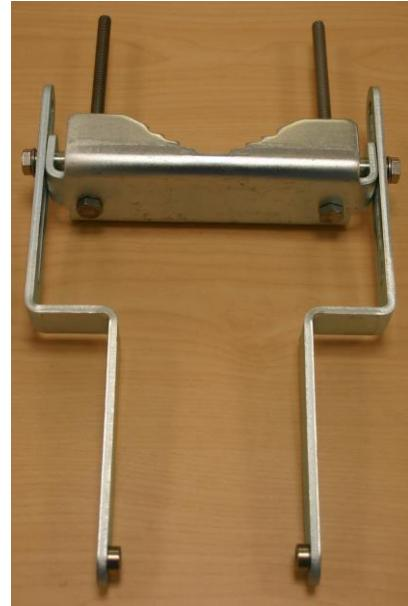
**4** Attach the rear strap to the bracket using (2) serrated flange nuts and (1) retaining bracket. Do not tighten the nuts now.
