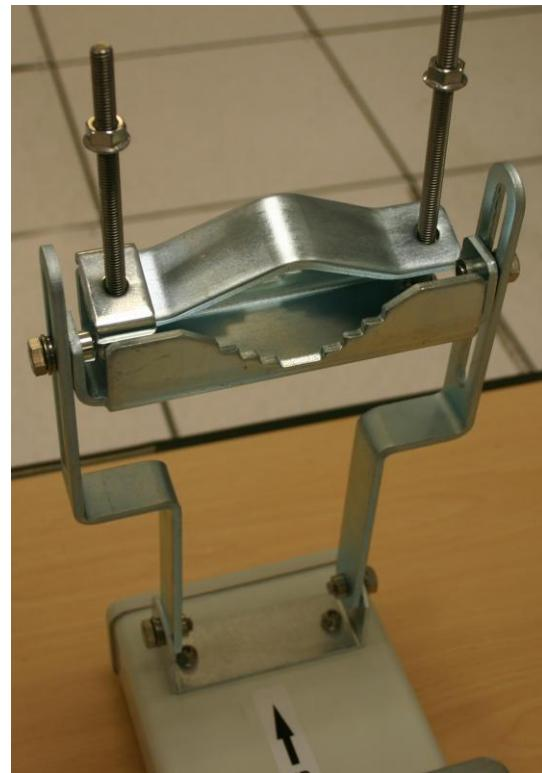
**6** Begin assembling the upper bracket by attaching the (2) 7" hex bolts to the bracket using (2) serrated flange nuts
