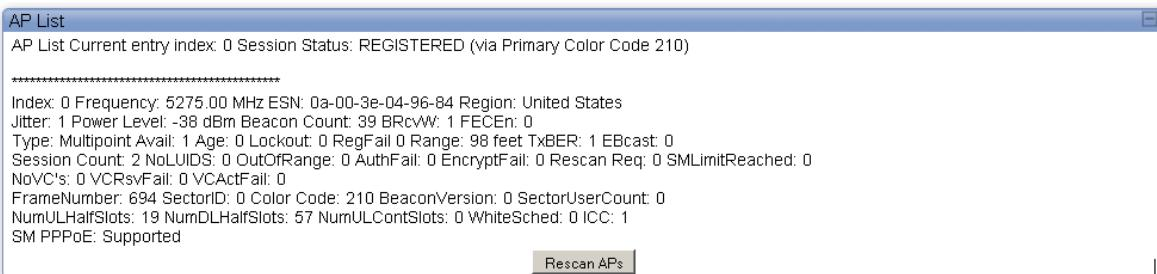
**Figure 29** SM Main Status - SM registered using primary Color Code 210
