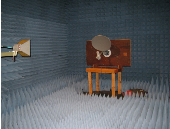
Radiated – Above 1 GHz - front
