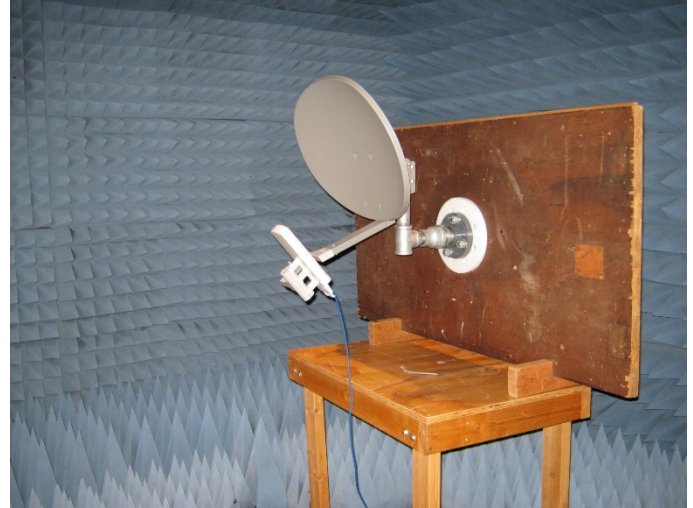
Radiated – Above 1 GHz - side
