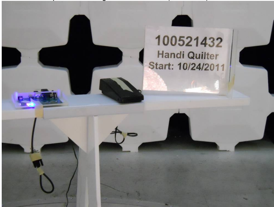
Base Test setup – Field Strength Measurements (Front View)
