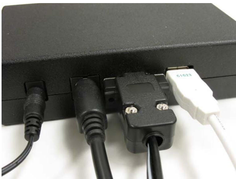
Installing the charging cable (may be black or white) into the HQ Sew Sweet™ Adapter
