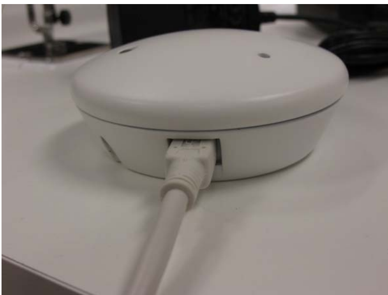
Charging cable installed. Note flat on cable is up.
