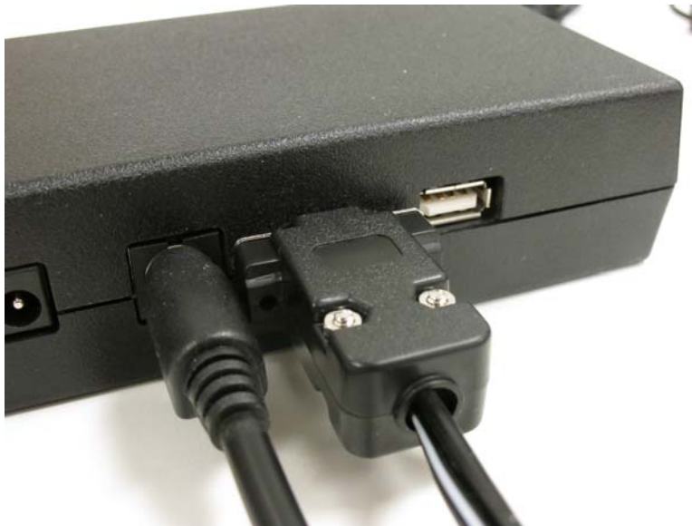
Installing the foot pedal (supplied with your machine) into the HQ Sew Sweet™ Adapter
