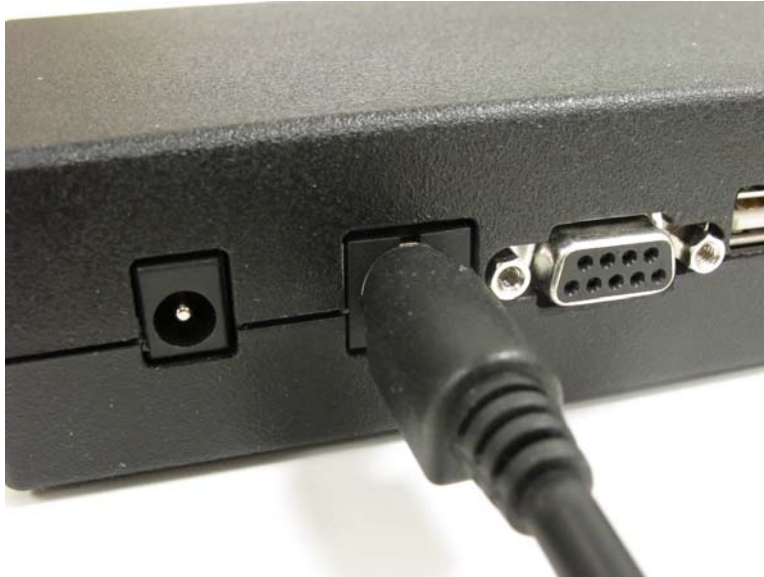
Installing the Machine Interface Connector into the HQ Sew Sweet™ Adapter
