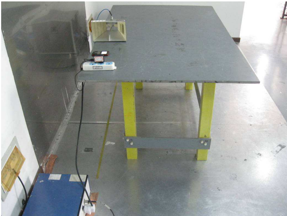
Conducted Emissions Test Setup - Side View
