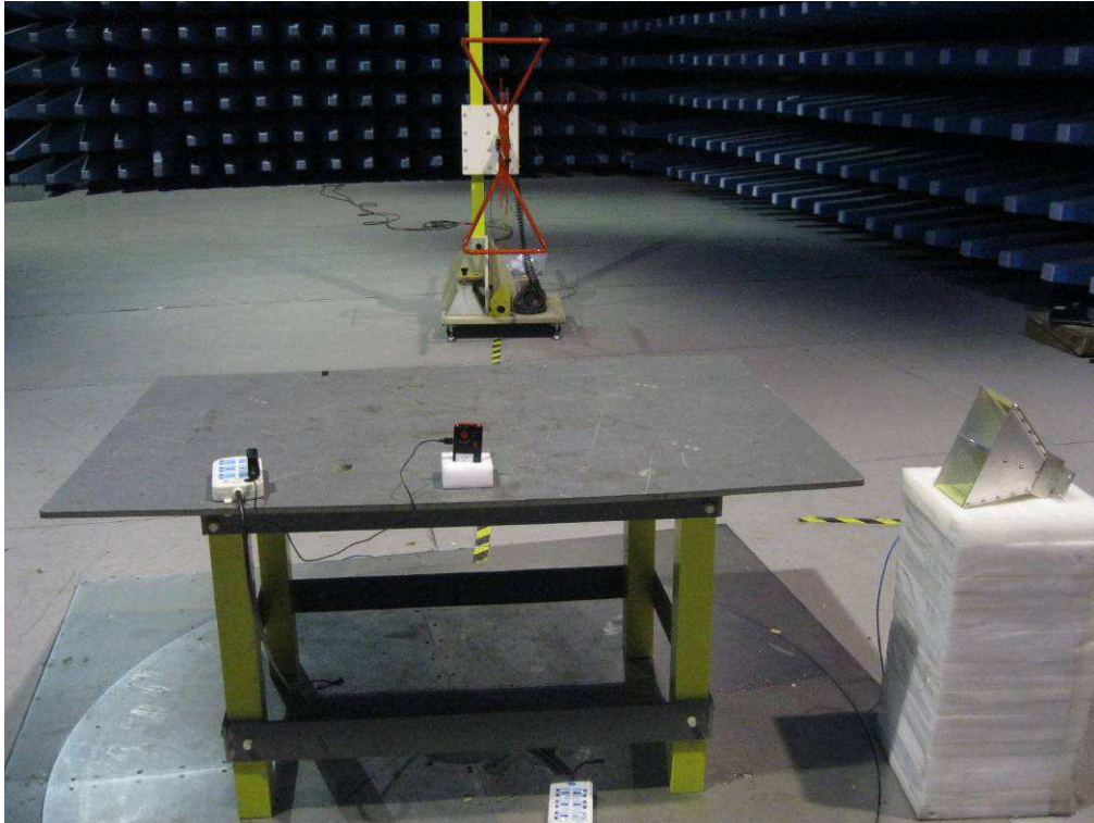
Radiated Emissions Test Setup Below 1GHz - Front View
