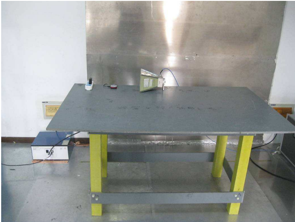
Conducted Emissions Test Setup - Front View
