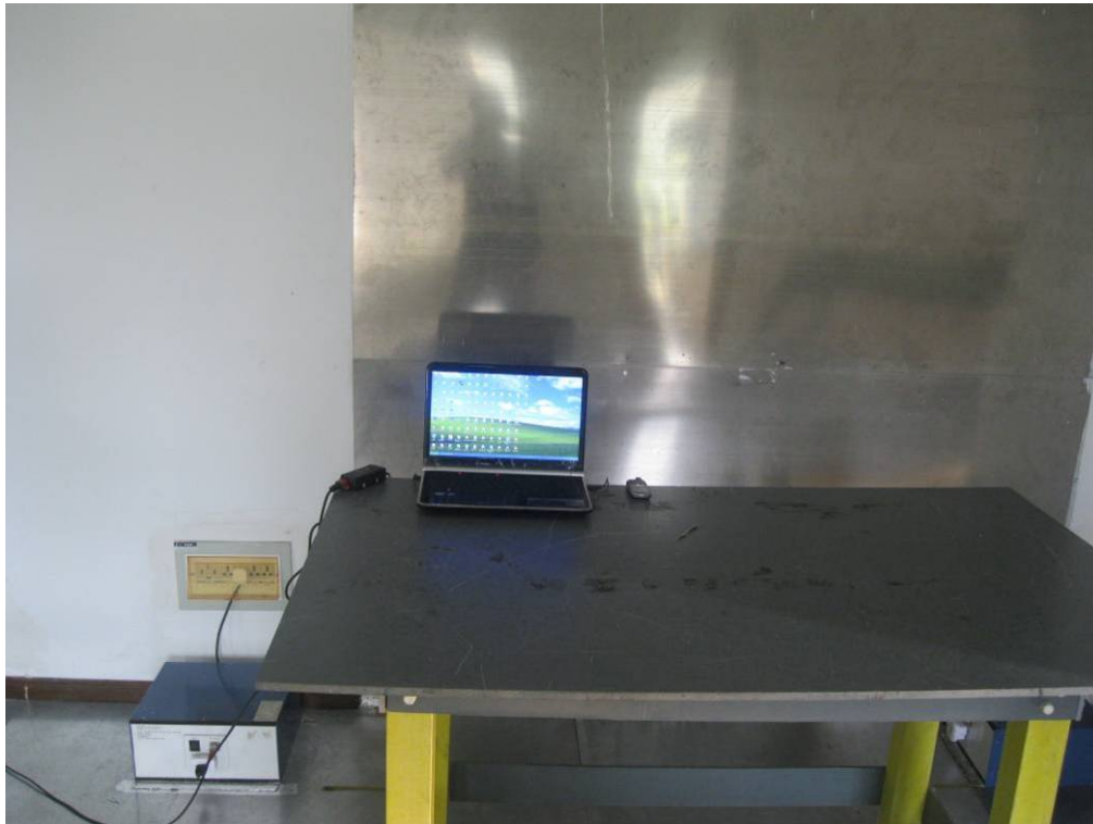
Conducted Emissions Test Setup Front View
