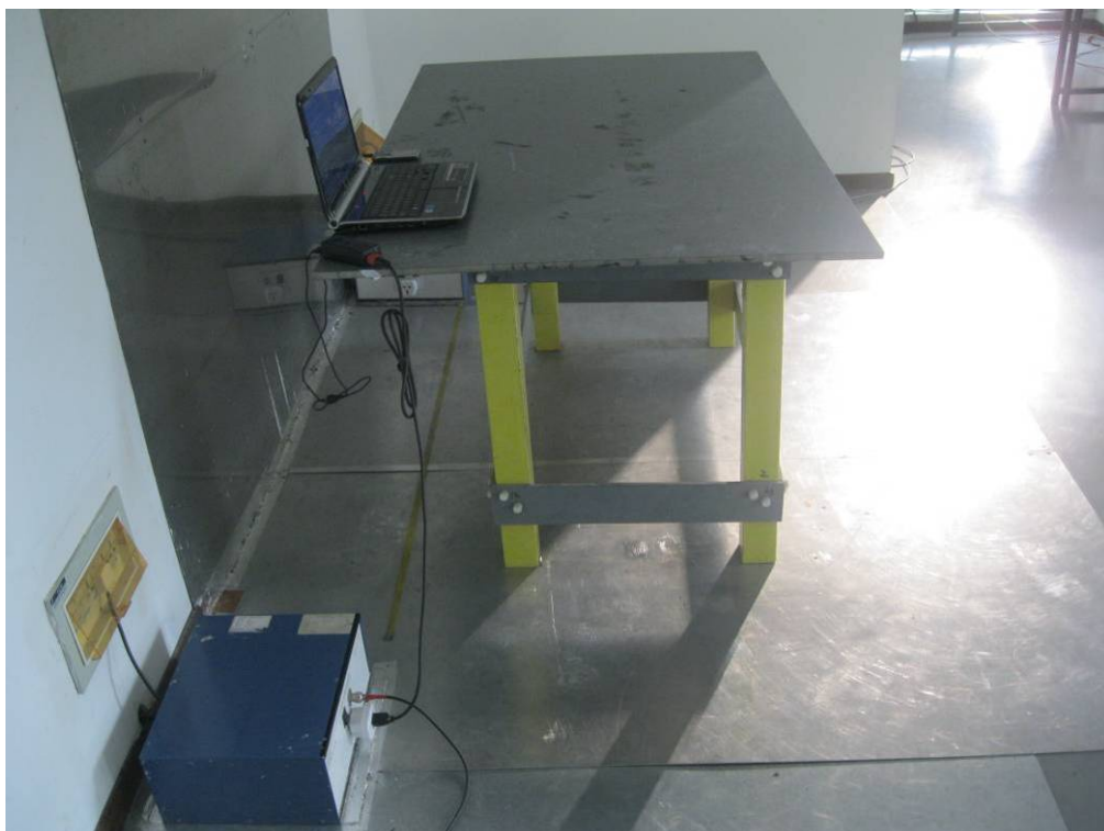
Conducted Emissions Test Setup Side View
