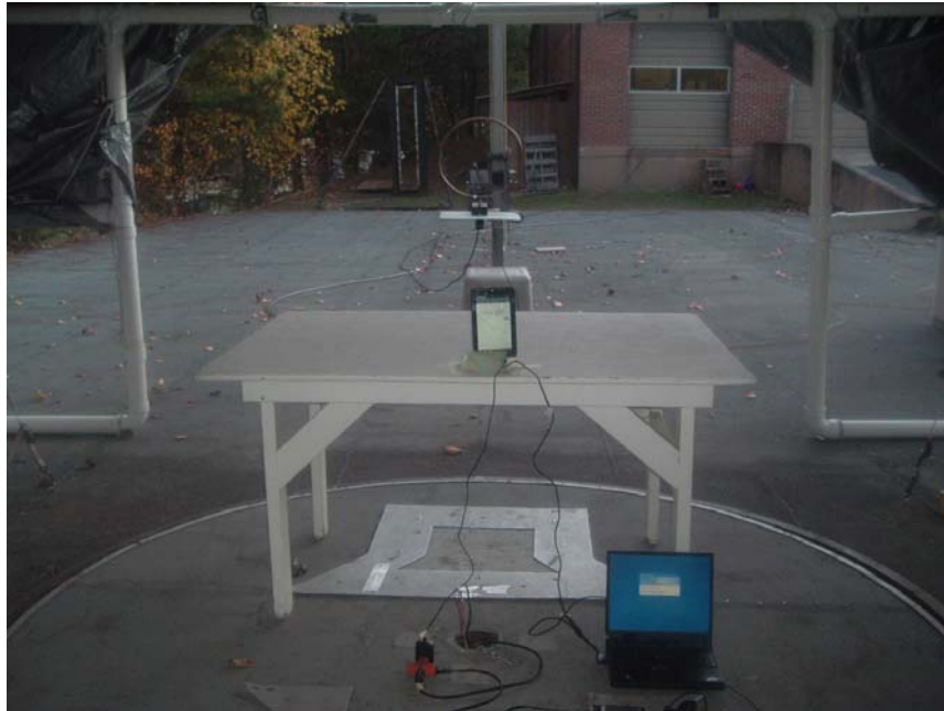
Figure 2- Test Setup from 1.705 MHz to 30 MHz
