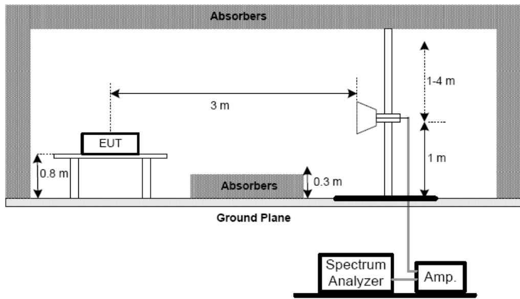
(C) For radiated emissions below 30MHz
