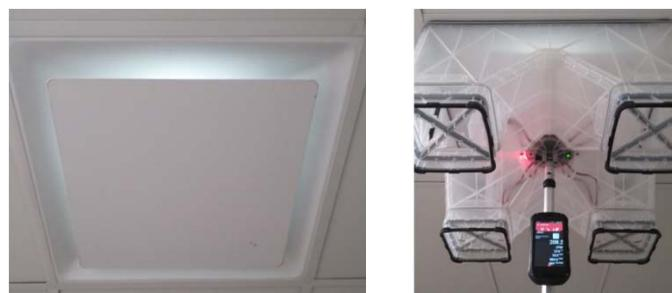
Once the SMART Air Hood™ is placed correctly, press the pole button to adjust the pole length so it reaches the floor supporting the hood itself. If the SMART Air Hood™ is not secure in place, readjust the pole length until it is more rigid.
