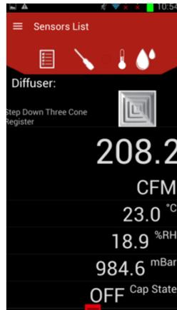
In order to read flow accurately, the correct diffuser style must be selected. To determine the diffuser style, look through the translucent body of the SMART Air Hood™ or remove the SMART Air Hood™ from the diffuser. In the below example, airflow is being measured from a *Plaque Register* diffuser style.
