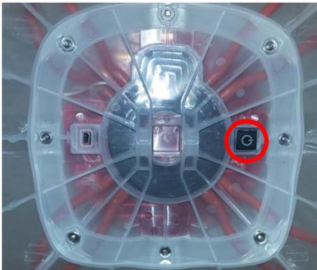
Once the SMART Air Hood™ is on, blue and red lights blink intermittently. This blinking pattern means that the SAH is not connected to its corresponding handheld device.
