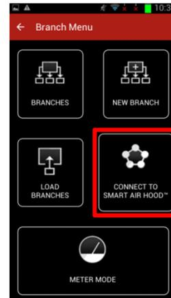
To connect to the SMART Air Hood™, tap the SEARCH button to locate it, and tap on the empty square of the found SMART Air Hood™ device.
