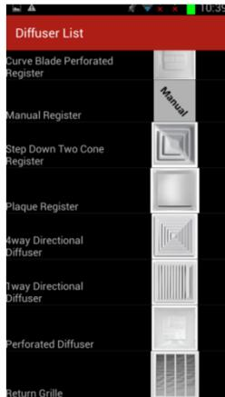
Tap on the appropriate icon to select that diffuser style, which in this example is the *Plaque Register*. Now the Plaque Register diffuser style is selected assuring accurate flow measurements.
