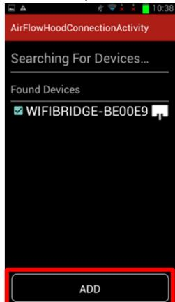
After adding the device, tap on the selected device. The following window pops up with the option to DELETE, CANCEL, or CONNECT. Tap on CONNECT so the handheld device can access data from the SMART Air Hood™, after which a waiting screen will show up and the red and blue LED lights will blink fast.
