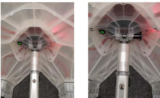
Attach the QUAD LOCK device on the handheld and the pole.
