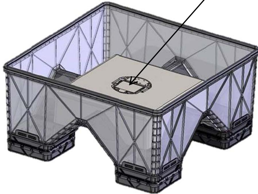
Label placement: external surface of battery cover as shown
