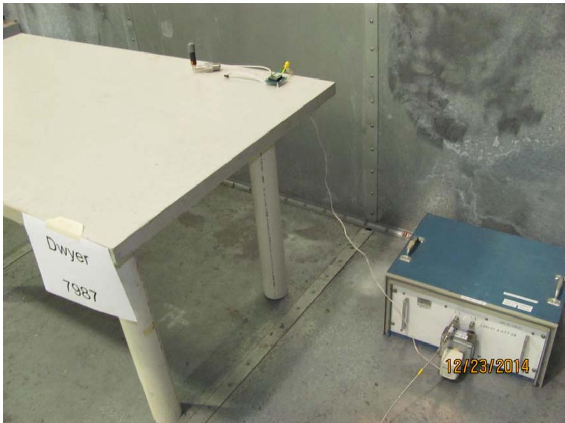
Photograph of Antenna Spurious Conducted Emissions Test Setup
