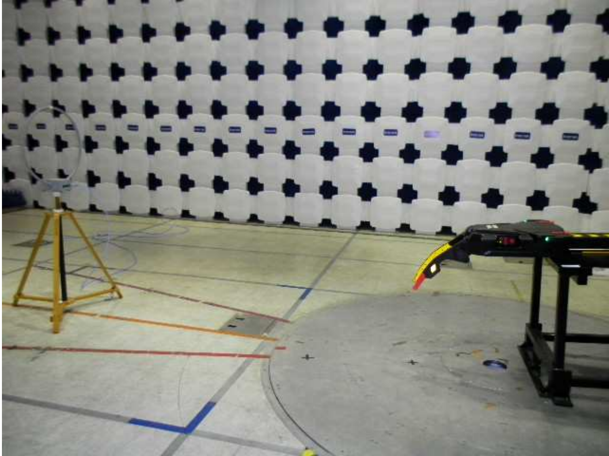
Fundamental and Offset Frequencies Test Setup Photo # 2
