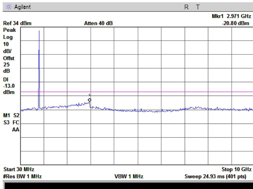
Conducted Emission Transmitting Mode CH 190
