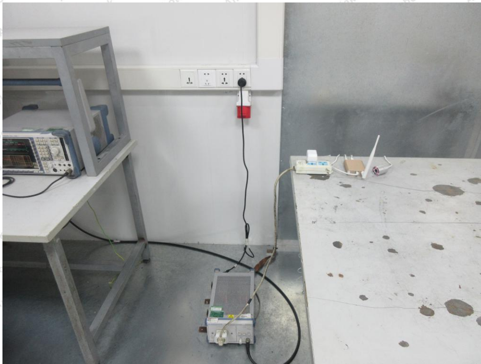
Photo of Conducted Emission Measurement
