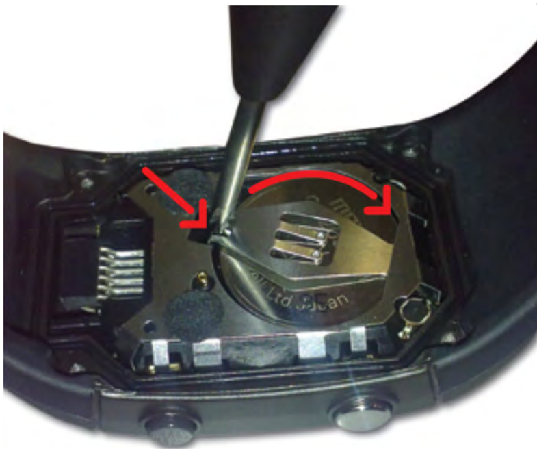
Figure 4-2. Removing Watch Battery
