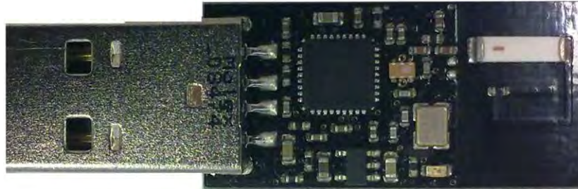
Figure 4-10. eZ430-Chronos RF Access Point
