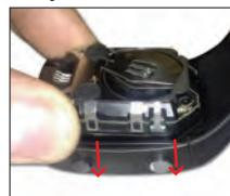
2. Ensure that metal strips on watch module slide over buttons.
