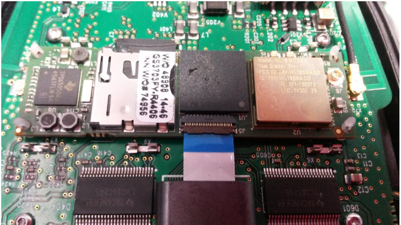
Photo 1: internal, Gumstix located on the display module
