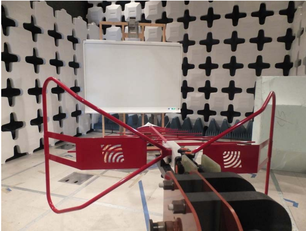
Figure 4.4A – Radiated Emissions 30M-1000M Test Setup - Front View
