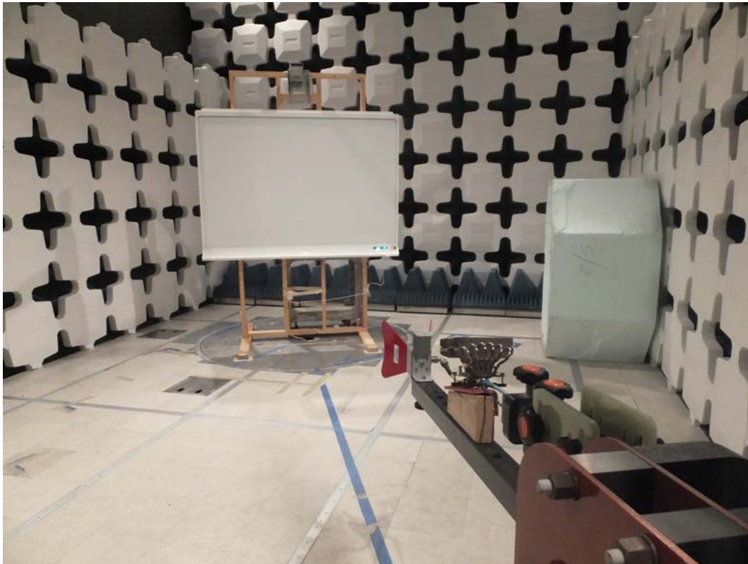
Figure 4.4C – Radiated Emissions 1G -18G Test Setup - Front View
