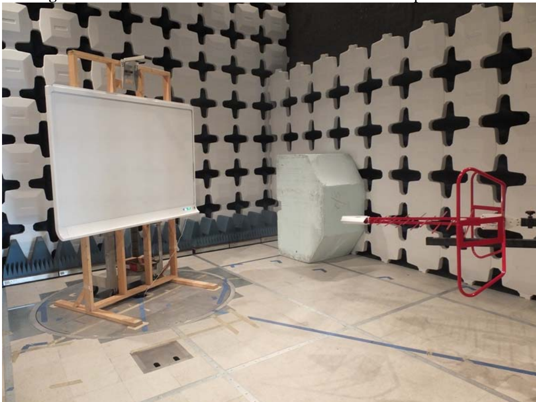
Figure 4.4B – Radiated Emissions 30M-1000M Test Setup - Side View
