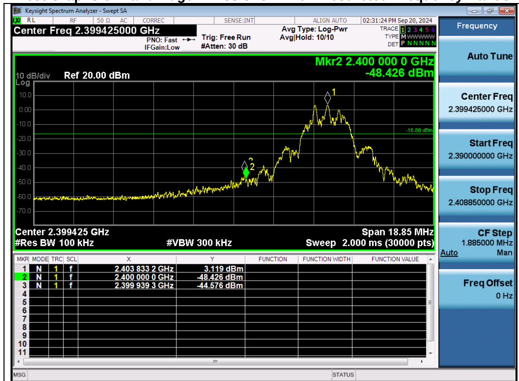
Test_Graph_2.4G_ANT1_2403.85_Lower Band Edge Emissions
