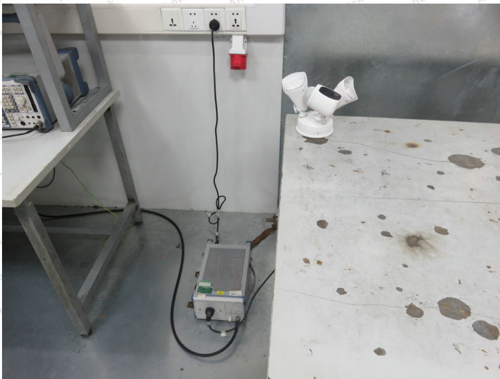
Photo of Power Line Conducted Emission Test
