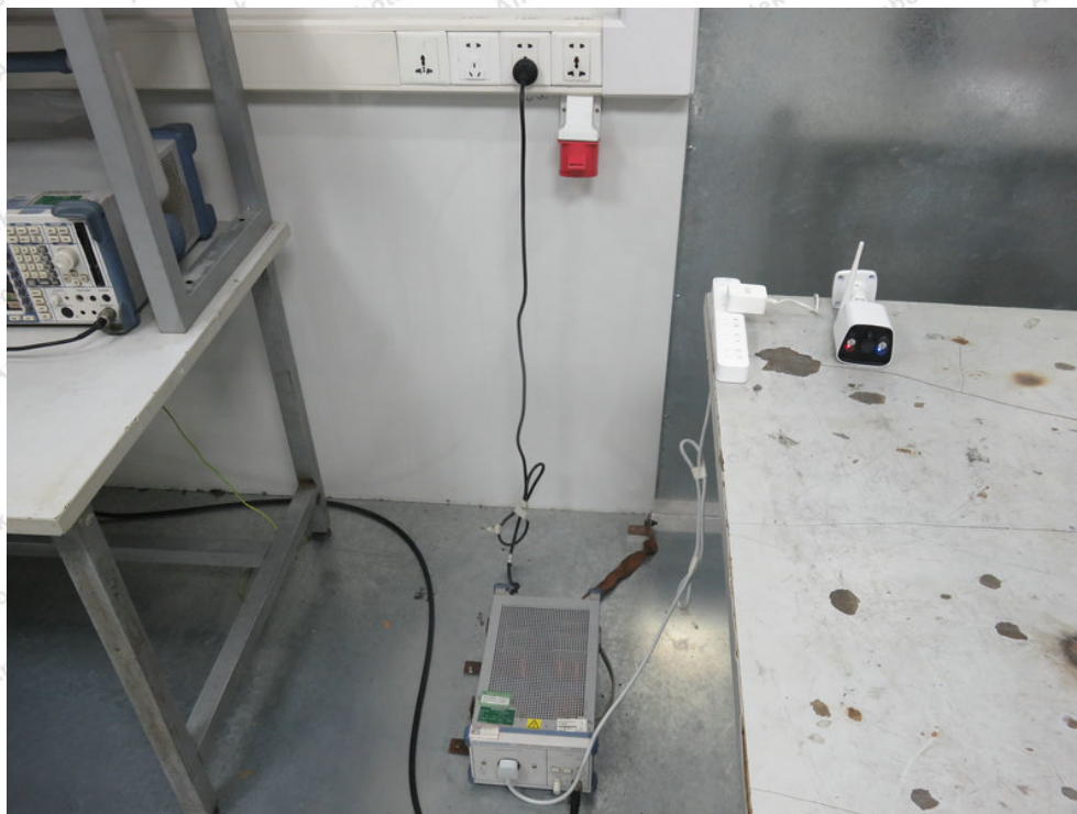
Photo of Power Line Conducted Emission Test
