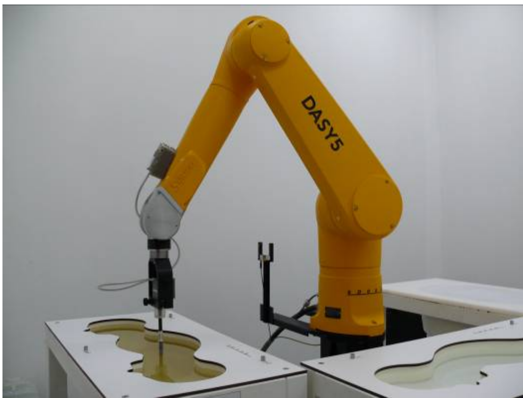
Picture 1: Specific Absorption Rate Test Layout
