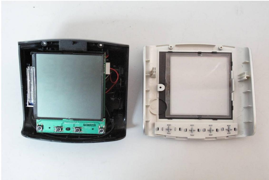
*Open View of EUT - 2 (TRICORE Crystal: 4MHz)*
