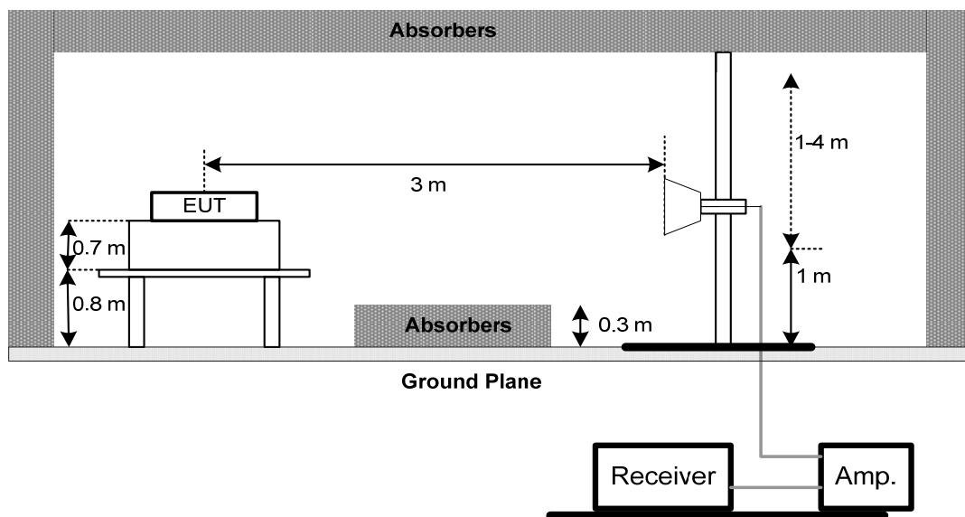
(C) For radiated emissions below 30MHz
