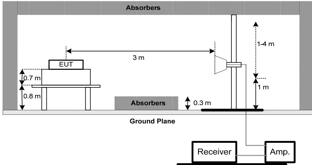
(C) For radiated emissions below 30MHz
