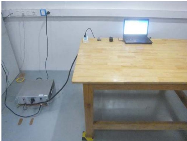
Conducted Emissions Test Setup Front View
