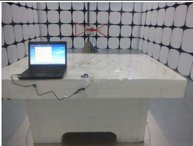
Radiated Spurious Emissions Test Setup Below 1GHz
