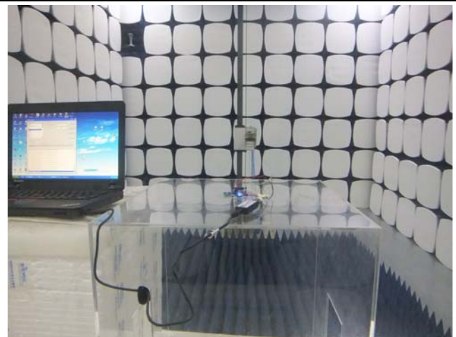
Radiated Spurious Emissions Test Setup Above 1GHz
