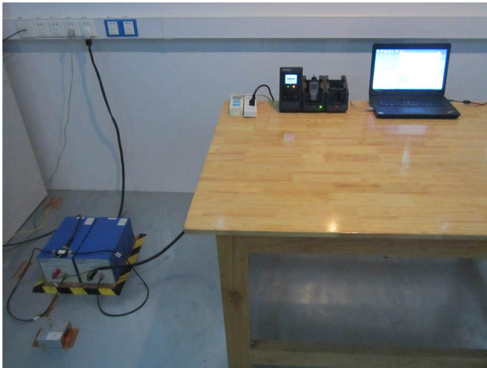
Conducted Emissions Test Setup Front View
