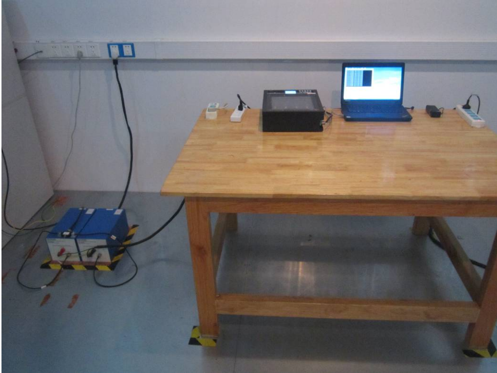
Conducted Emissions Test Setup Front View
