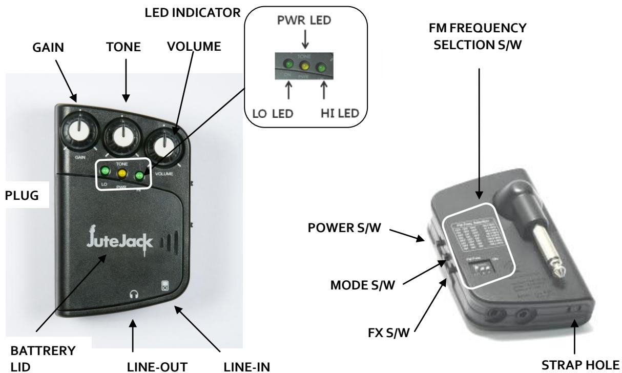
**GAIN:** Gain control knob for distortion
