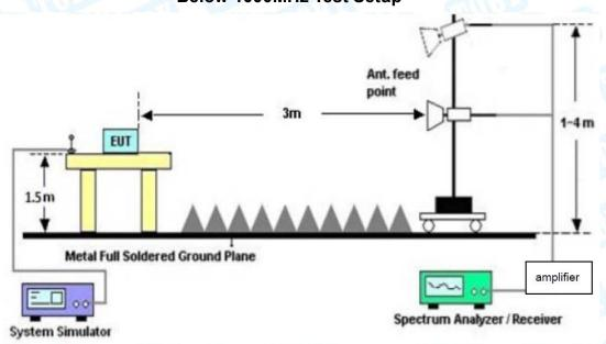
**Above 1GHz Test Setup**
