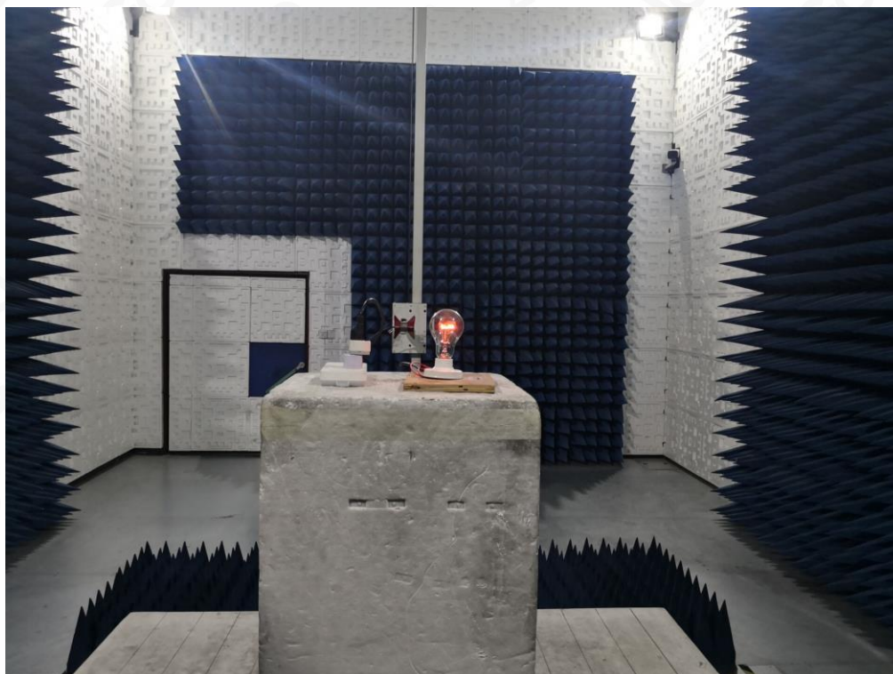
FCC RADIATED EMISSION TEST SETUP ABOVE 1GHZ
