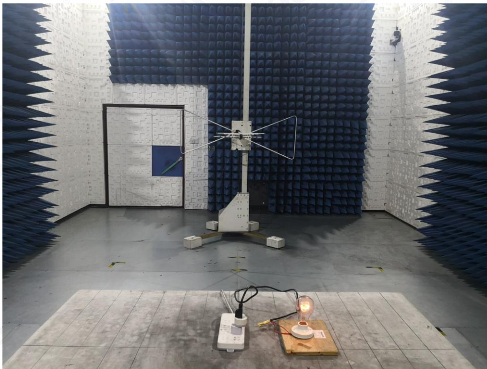
FCC RADIATED EMISSION TEST SETUP ABOVE 1GHZ
