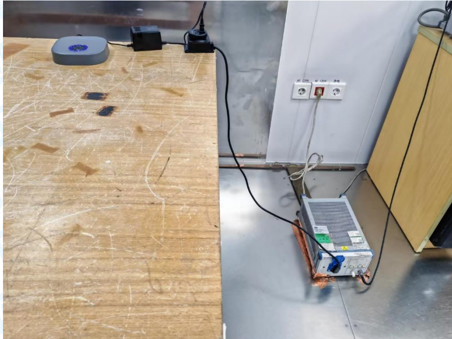
Photo of Setup for Radiated Emission (30MHz~1GHz)
