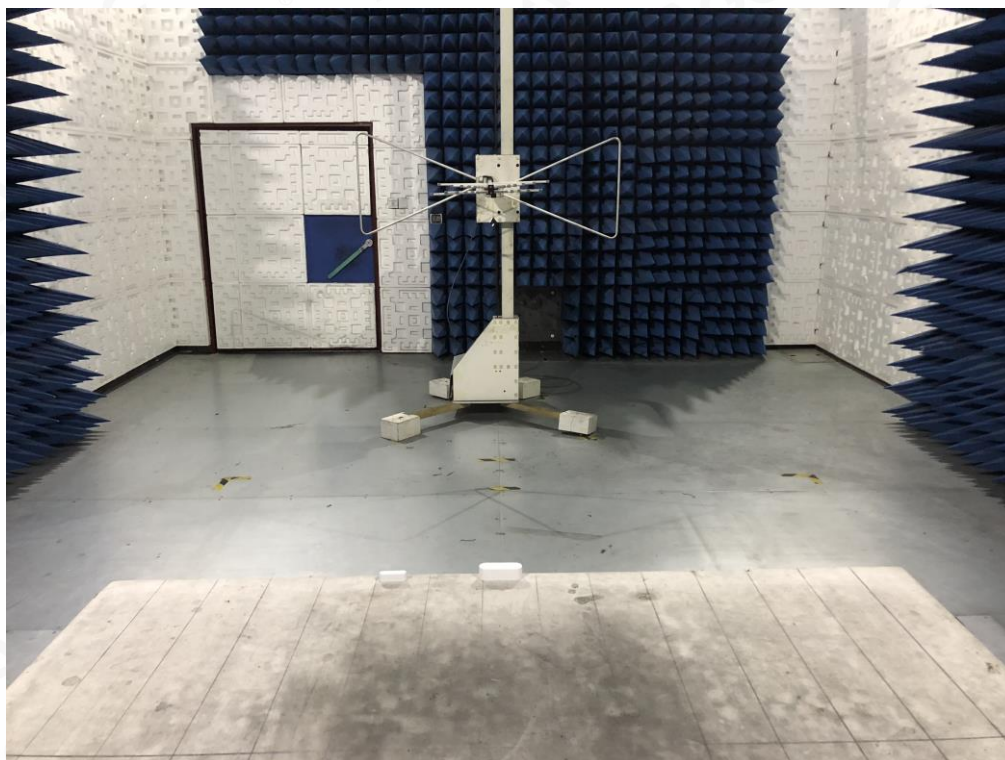
FCC RADIATED EMISSION TEST SETUP ABOVE 1GHZ
