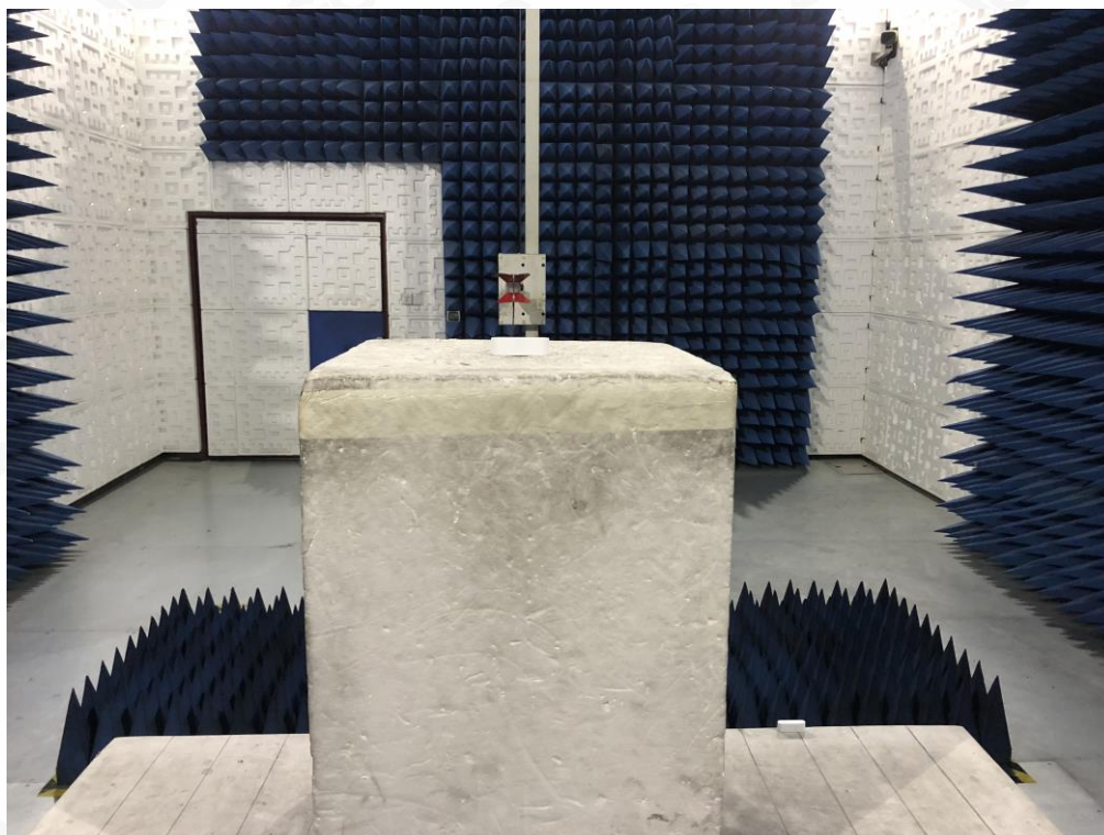
FCC RADIATED EMISSION TEST SETUP ABOVE 1GHZ
