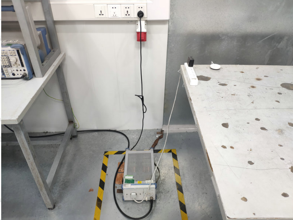
Photo of Power Line Conducted Emission Test
