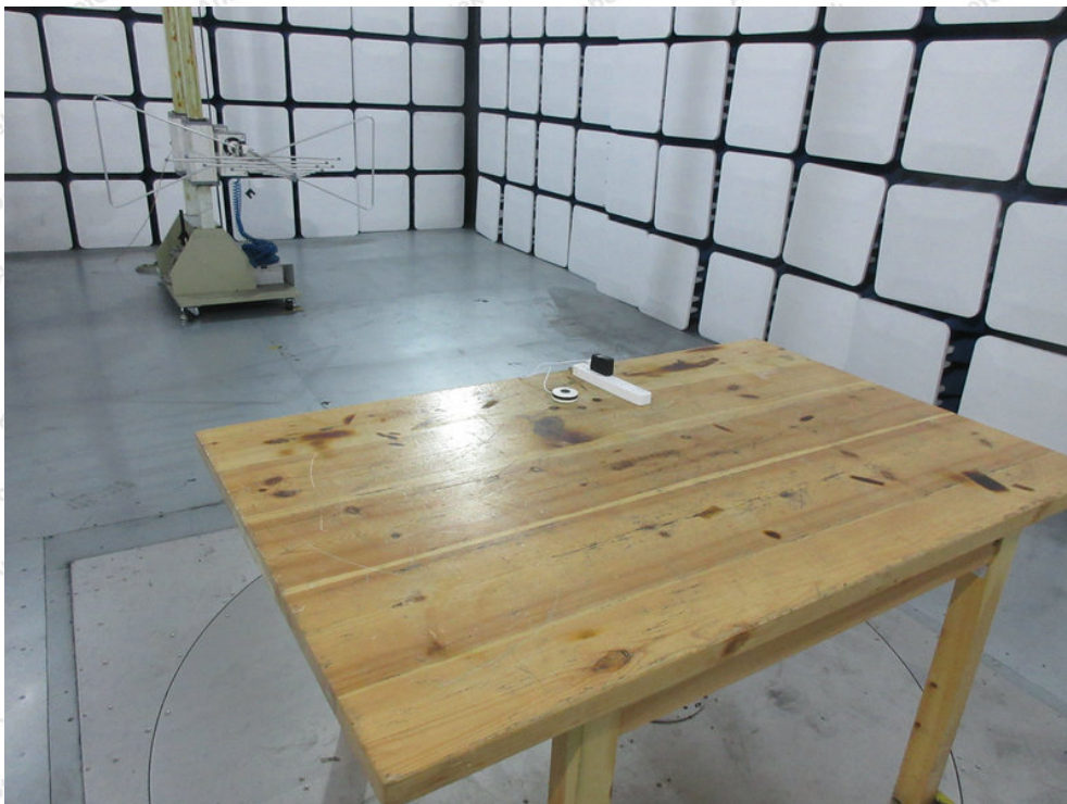
Photo of Radiation Emission Test
