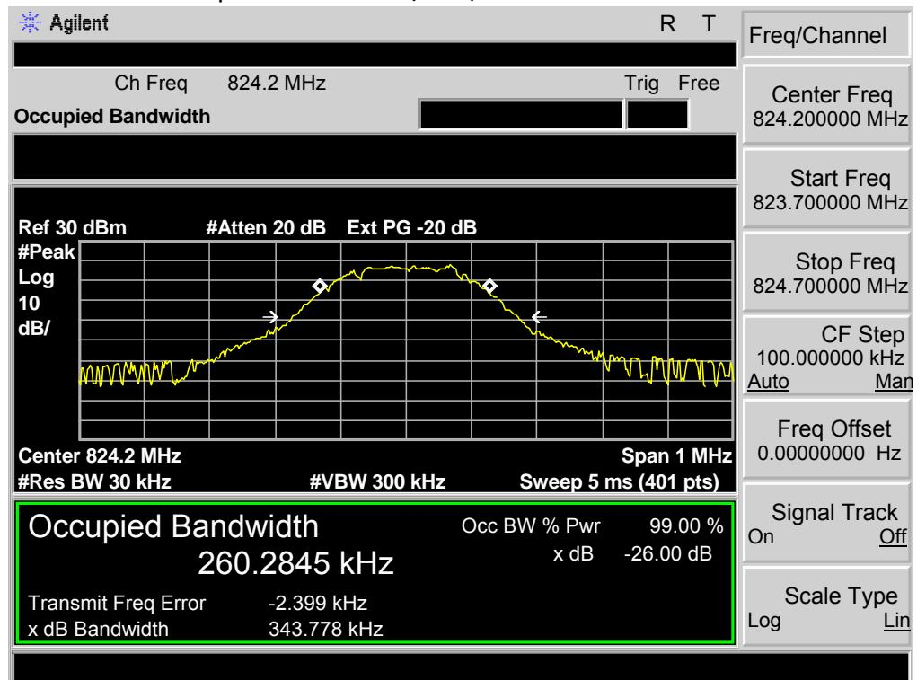
Occupied Bandwidth (99%) GSM 850 BAND CH 190
