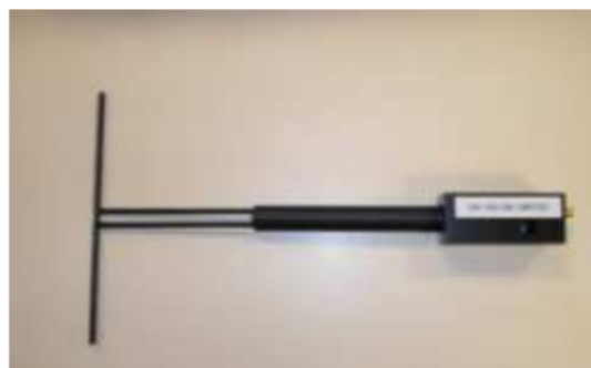
Figure 1 – Satimo COMOSAR Validation Dipole
