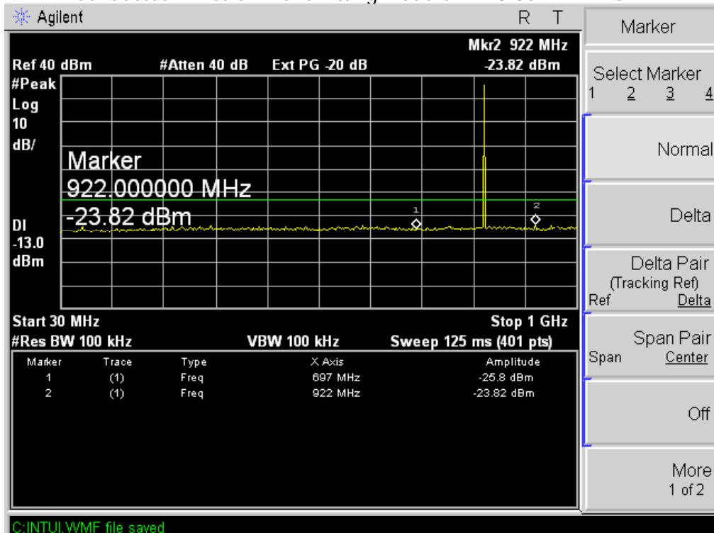
Conducted Emission Transmitting Mode CH 128 30MHz – 1GHz
