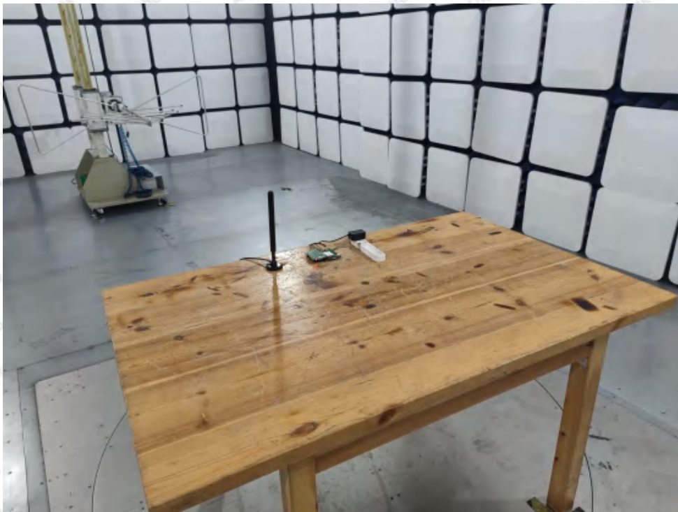
Photo of Radiation Emission Test
