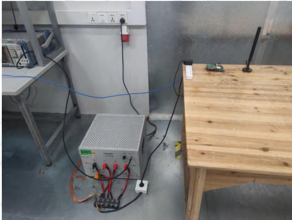
Photo of Conducted Emission Measurement
