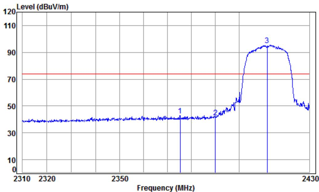
Mode:b; Polarization:Horizontal; Modulation:802.11n; bandwidth:20MHz; Channel:Low
