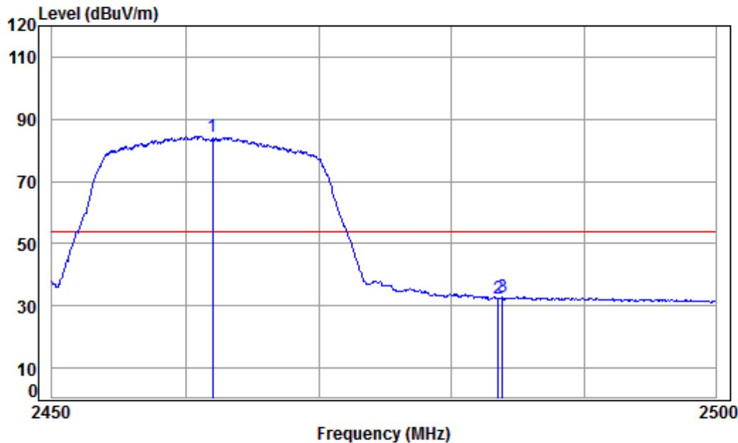
Mode:b; Polarization:Horizontal; Modulation:802.11n; bandwidth:20MHz; Channel:Low
