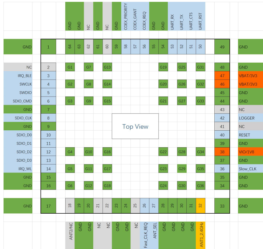
Figure 2-3. BM3301-1313 Module Pin arrangement
