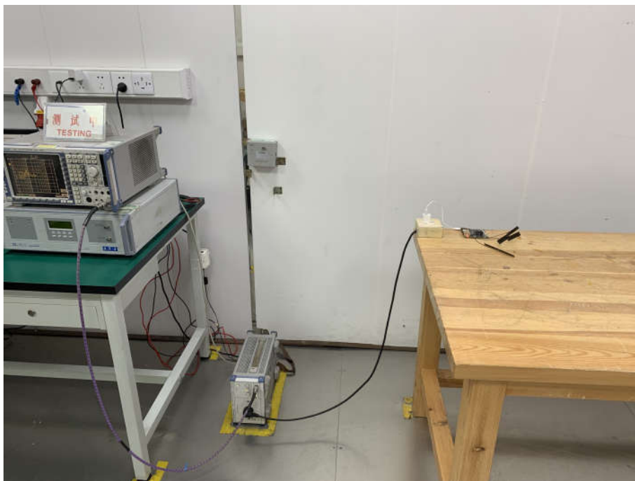
Conducted Emissions Test Setup
