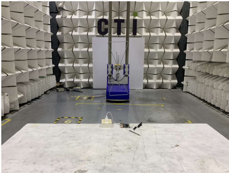
Radiated spurious emission Test Setup-1(Below 1GHz)
