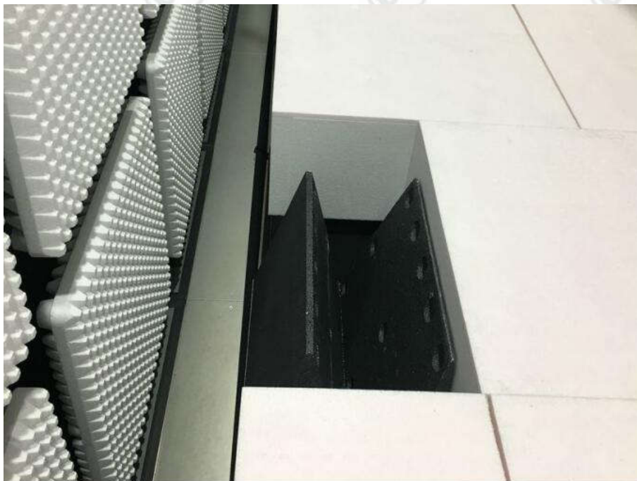
Radiated spurious emission Test Setup-3(Above 1GHz) There are absorbing materials under the ground.
