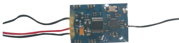
This 2,4GHz features a unique coding protocol, to use this transmitter with a receiver it must be bound to the receiver. The factory will bind the transmitter to the receiver but should it become unbound or should you purchase a second receiver then please follow the procedure outlined below.
