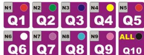
**Fixture Select buttons** are multi function buttons. The will be used to select a fixture, Change networks and select a color preset.
