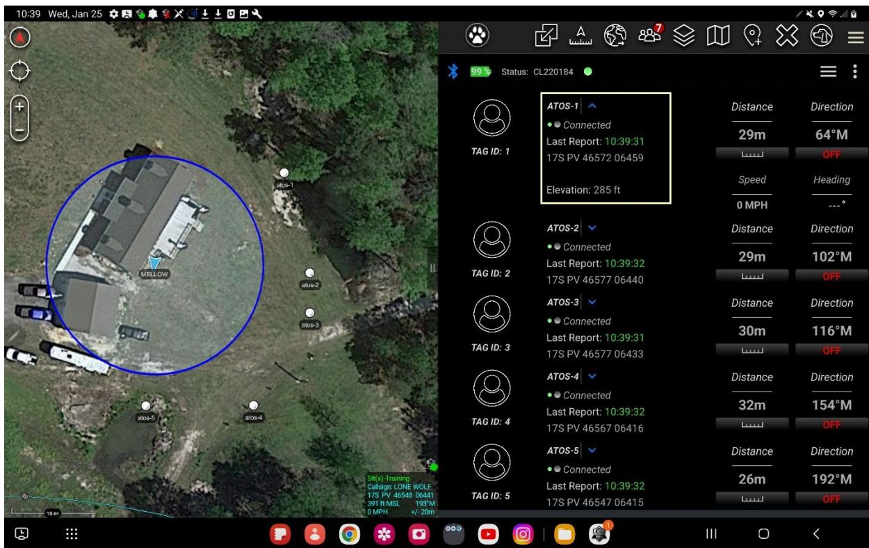
The ATOS plug-in will display the status of the command link connection.
