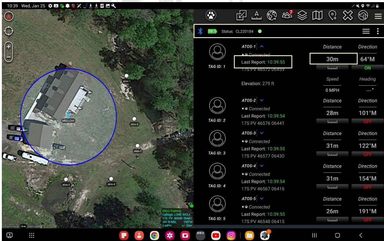
ATOS Command Link will start “SCANNING” and connect, then display serial number of the paired CommandLink “CLXXXXXX”. A green light indicator and battery % will show Status of CMND Link.
