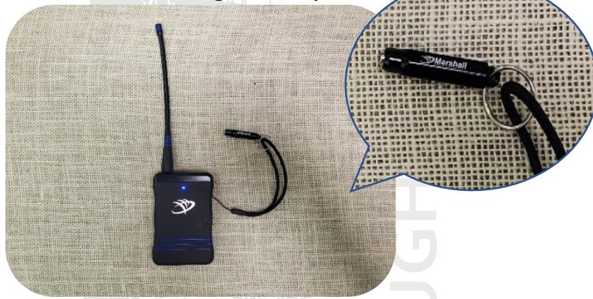
Place the key to the power symbol at the top of the CommandLink for 1 second. Three audible beeps and three purple flashes indicate a successful power up. Note: if the key is held to the power button too long the CommandLink may turn off. Bootup time, approx. 20s.
