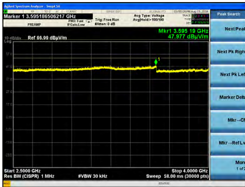
Channel 39, Vertical Orientation, Antenna Vertically Polarized, 2500 MHz to 4000 MHz, Reduced VBW
