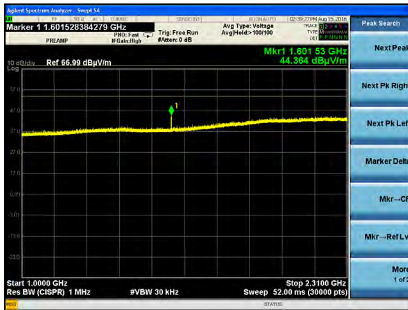
Channel 19, Vertical Orientation, Antenna Vertically Polarized, 1000 MHz to 2310 MHz, Reduced VBW
