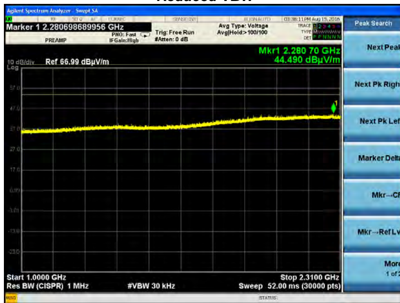
Channel 19, Vertical Orientation, Antenna Vertically Polarized, 1000 MHz to 2310 MHz, Reduced VBW
