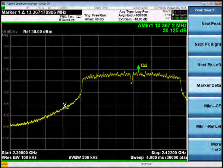
Screen Capture Demonstrating Compliance at the Lower Band-Edge
