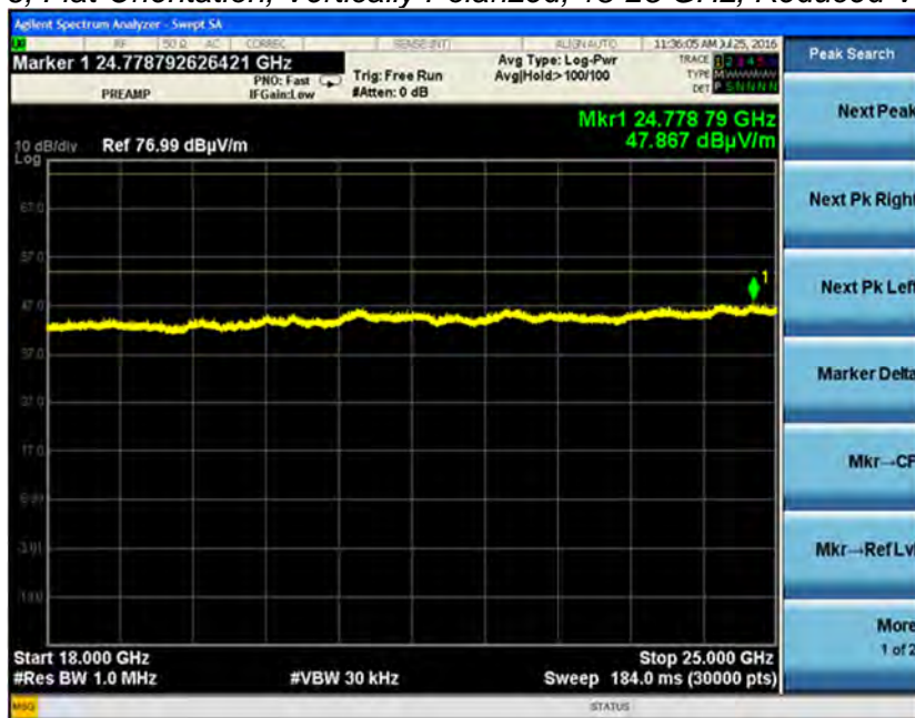
Channel 6, Flat Orientation, Vertically Polarized, 18-25 GHz, Reduced VBW at 3m
