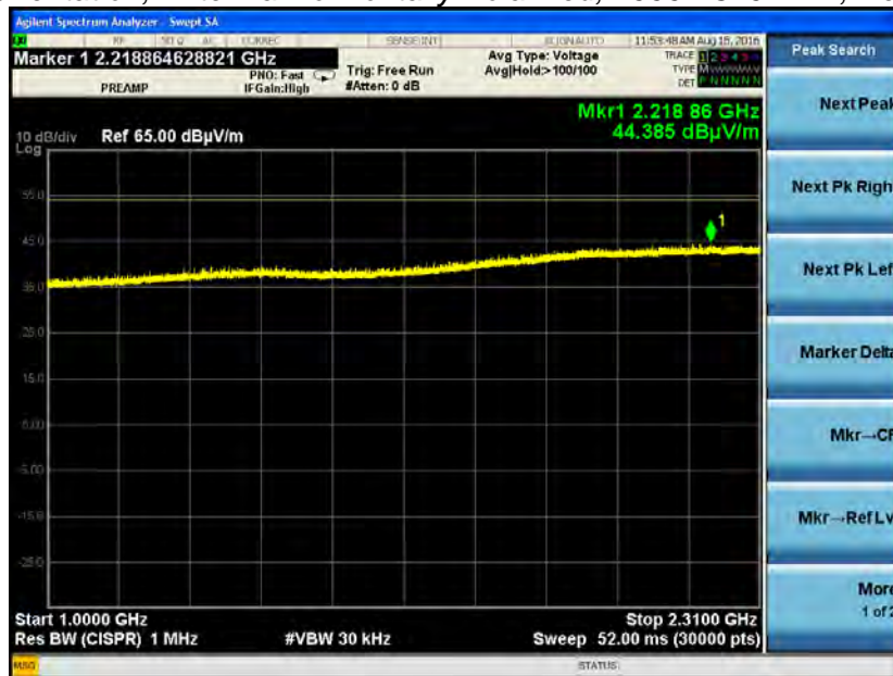
Channel 1, Flat Orientation, Antenna Horizontally Polarized, 1000-2310 MHz, Reduced VBW at 3m
