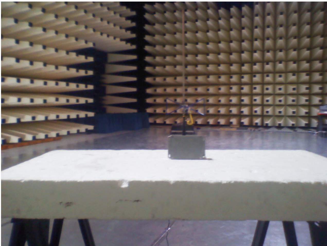
Figure 1: Radiated emissions setup below 1 GHz
